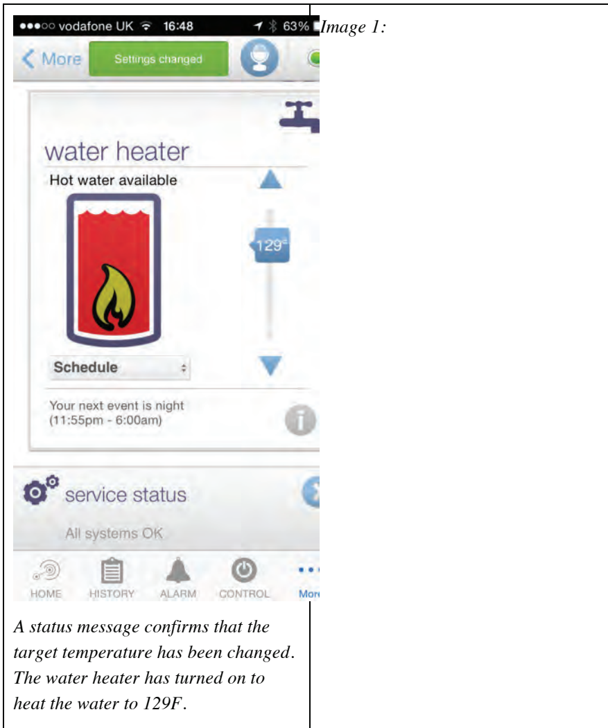
Figure 9.30: The Lowes Iris water heater UI, showing the status message
