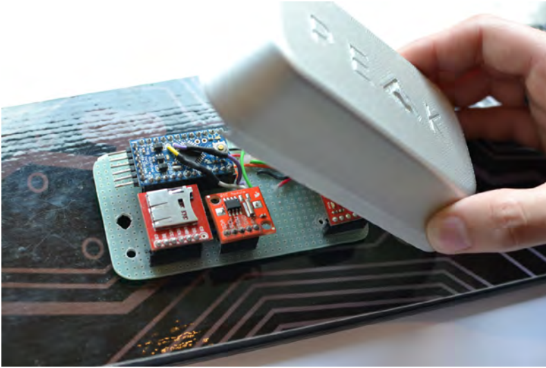
Figure 14-2. A higher fidelity prototype of the electronics and enclosure for the skis 3
