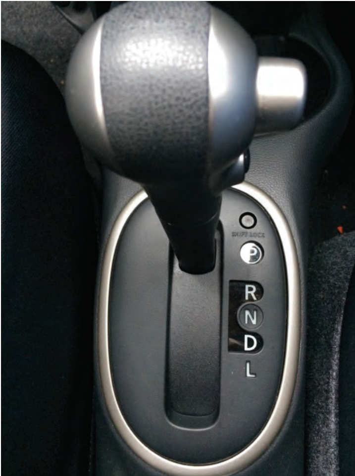
Figure 9.10: automatic gearbox controls hide the complexity of the system behind a simplified conceptual model
