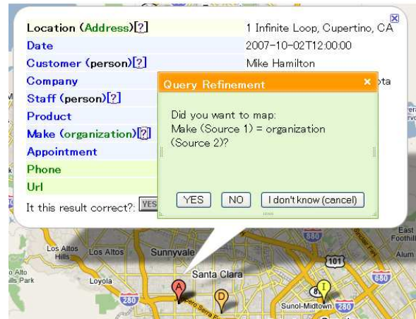
Figure 5: Decision-level feedback: the popped dialog window shows mapping between attributes (“Make” and “organization”) in two sources, which is used as a join condition. The user can answer whether this mapping is correct.
