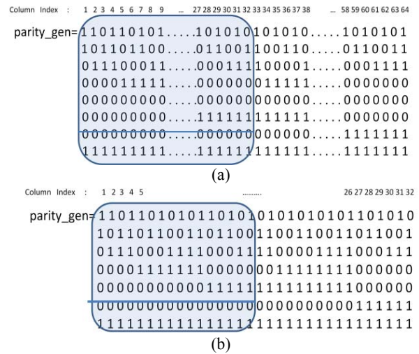
Figure 6: a) Parity generation of (39, 32) code from (72, 64) code, b) Parity generation of (22, 16) code from (39, 32) code
