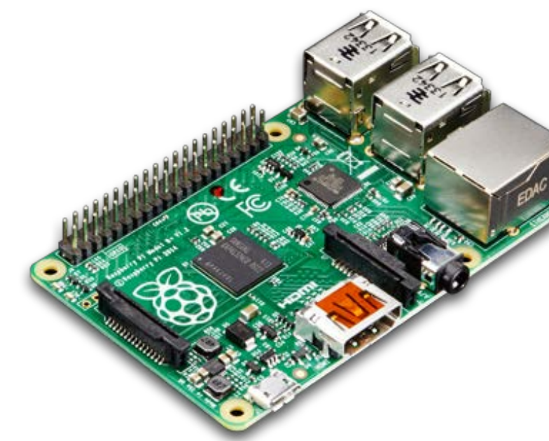
Figure 2: A Raspberry Pi Computer Board
