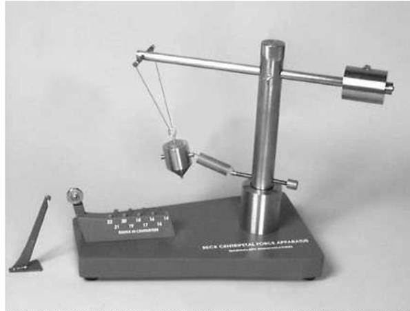
You will be asked to perform five trials of this experiment. For the first three trials, keep the circle radius fixed and use three different values of the mass of the moving object. For the last two trials, use two new values for the circle radius. For each trial, you will have to make three separate measurements of the time for 30 revolutions and take the average of those three. Here is the procedure for each of the five trials.
