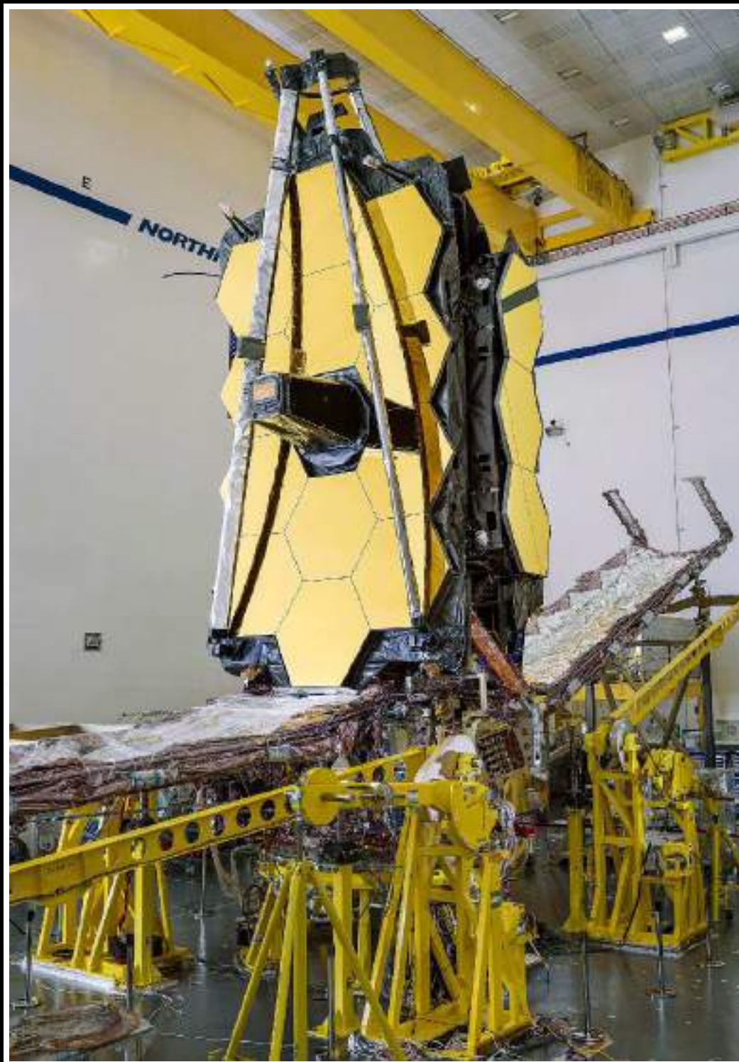
August 2019: JWST OTE+ISIM integrated with Sunshield+Spacecraft!
