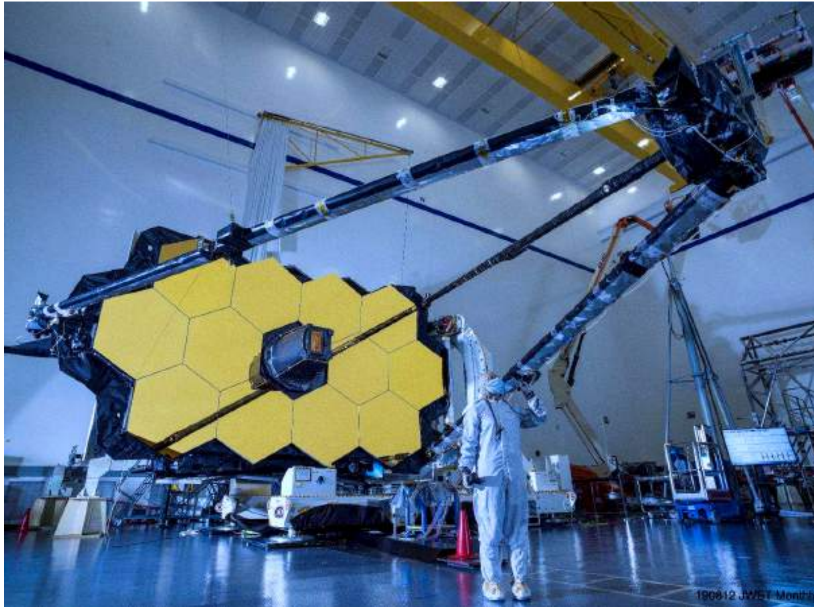
Aug. 2019: OTE before final integration with Sunshield & spacecraft.
