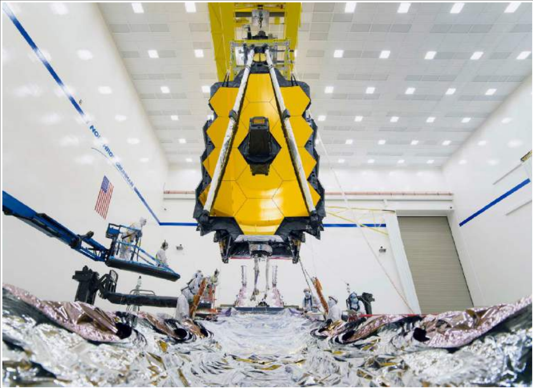
August 2019: JWST OTE+ISIM lowered into Sunshield+Spacecraft
