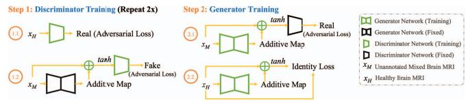
Figure 2. A training iteration in Brainomaly involves two steps: (1) the training of the discriminator and (2) the training of the generator. The discriminator is taught to identify the difference between real images and those generated by the generator. Meanwhile, the generator attempts to create indistinguishable images from real images to trick the discriminator. The iteration is repeated multiple times during the training phase to improve the realism of the generated images.
