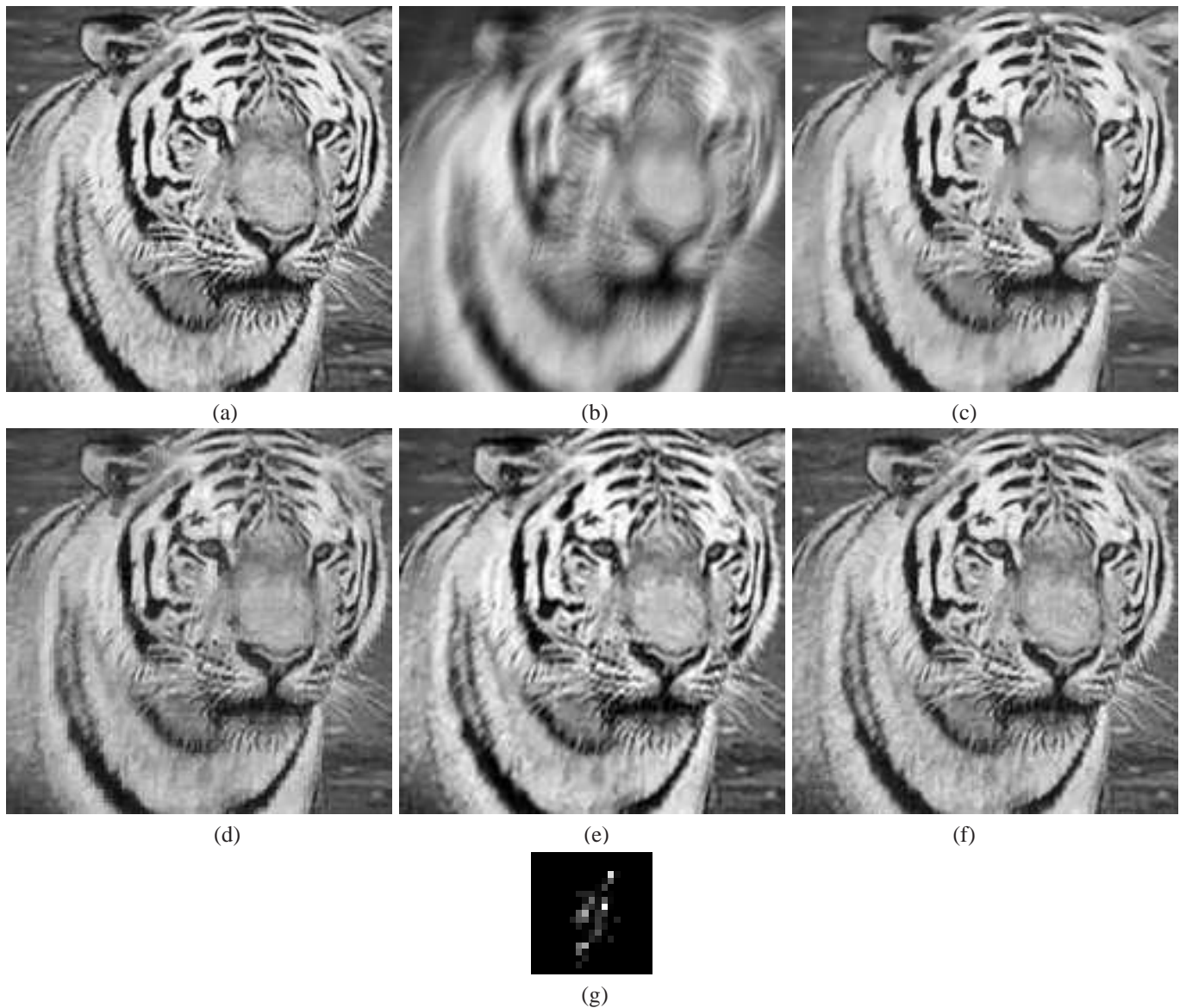
Fig. 6. Details of the image deconvolution experiment with a Tiger image. (a) Original image. (b) Noisy blurred image. (c) Hyper-laplacian [37] estimate (ISNR 8.14 dB). (d) Wavelet domain sparsity-based estimate [9] estimate (ISNR 8.28 dB). (e) LPA-ICI [23] estimate (ISNR 9.14 dB) (f) Parametric manifold-based estimate suggested in this paper (ISNR 9.02 dB). (g) Blur kernel.
