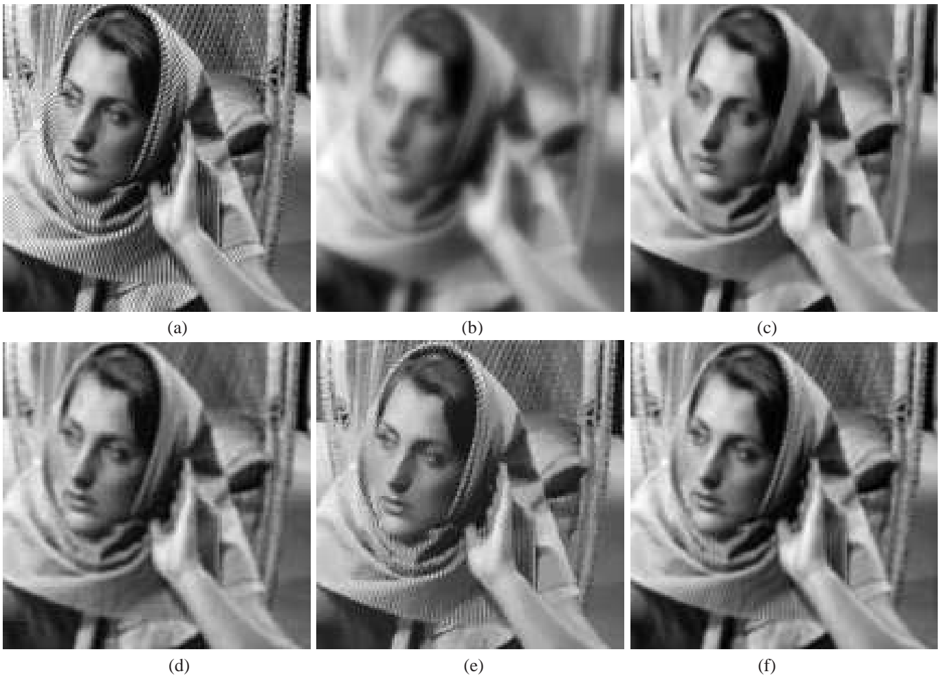
Fig. 5. Details of the image deconvolution experiment with a Barbara image. (a) Original image. (b) Noisy blurred image. (c) Hyper-Laplacian [37] estimate (ISNR 5.19 dB). (d) Wavelet domain sparsity-based estimate [9] (ISNR 6.24 dB). (e) LPA-ICI [23] estimate (ISNR 7.88 dB) (f) Parametric manifold-based estimate (ISNR 7.98 dB) suggested in this paper.
