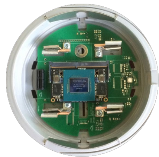
Smart grid chip with GPU for edge computing and AI
